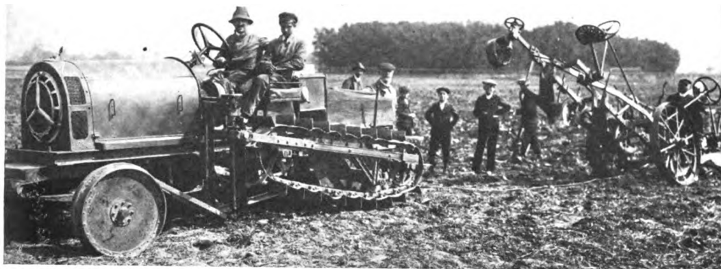
Above—Lefebvre caterpillar tractor hauling double-ended plow. Below—Case tractor at the Grigny demonstration
